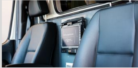
The UX10-IP tablet in the rescue vehicle permanently attached to the Havis vehicle dock.
